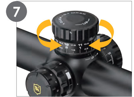
Zero in your scope to achieve the desired zero stop shooting distance (e.g., 200m/yds) by adjusting the elevation turret up or down as needed
